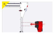
> Present the fall arrest block to the Upright as shown and ensure it is aligned with the holes
