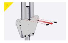
While in this vertical position remove ball lock pin from its stow hole on the Trap Plate.
