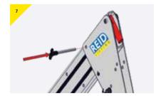
Re-insert ball-lock pin into hole ensuring the pin is fully engaged through hole. A gentle rocking motion can be used to induce alignment
