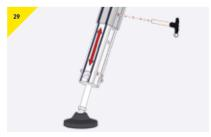
> For coarse adjustment in leg height set cartridge at desired point (2x50mm increments)
